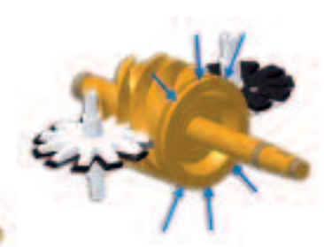
Radial loads act on both the top and underside of the main rotor.
